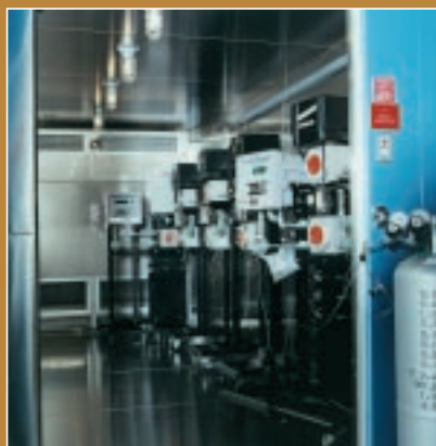
Daniel GC's must pass a rigid operational test with on-line calibration standards in environmental chambers at temperatures from 0° to 130°F. Daniel dependability results from our dedication to in-house testing and quality control.
